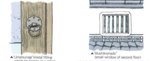
▲"U Matsunagi"(metal fitting which tie horses to a pillar) ▲"Mushikomado"(small window of second floor) Mushikomado is the grid style plastered window which look like insect cage. There are the various design windows in Seki Juku.
